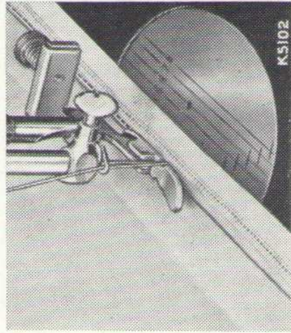
Fig. 71. Cording Foot (At left of needle). Applying Fold to Zipper Tape.
