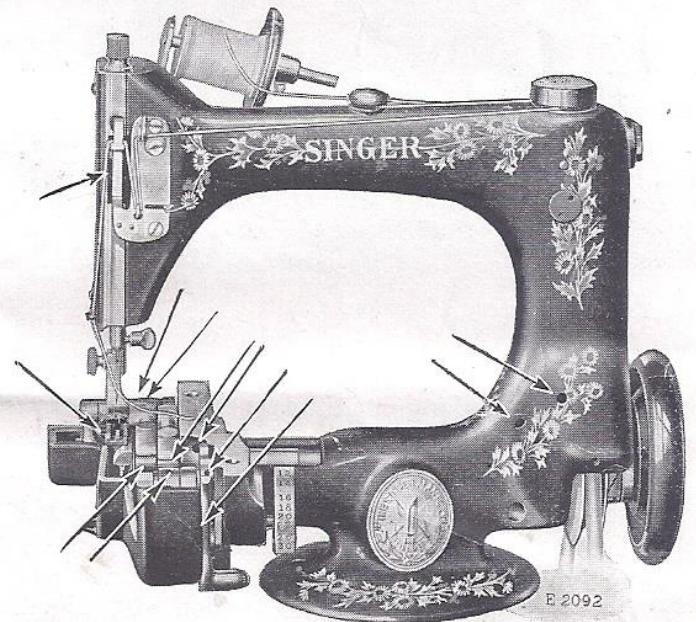
FIG. 9. OILING POINTS AT THE FRONT OF THE MACHINE
