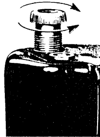
Fig. 27. Regulating Pressure on the Material
